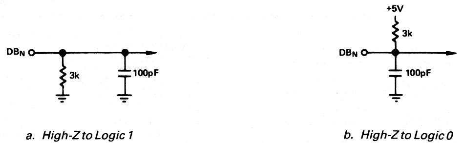
Figure 4. Load Circuit for Access Timing Test
