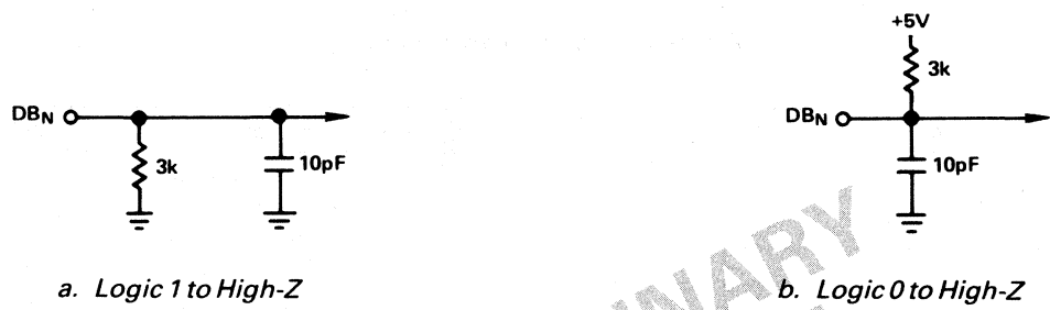
Figure 5. Load Circuit for Output Float Delay Test
